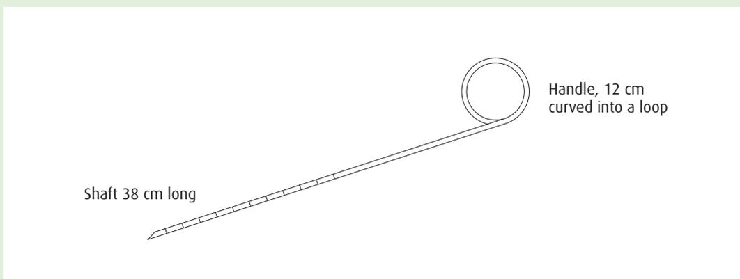
Metal rod (50 cm long, 3.15mm diameter) with file marks every 2.5 cm starting from end of rod.
